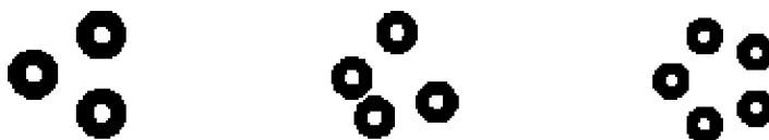
Figure 3. Optimal aperture configurations with 3, 4 and 5 elementary telescopes, for a given collecting surface and resolution.
