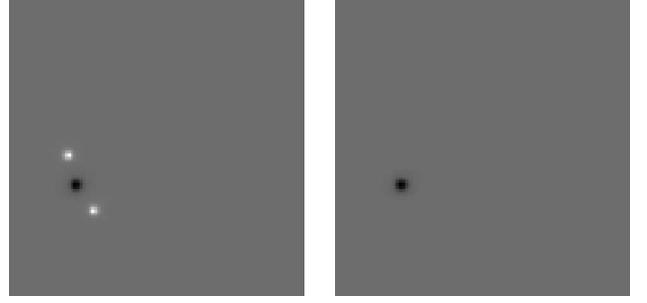
Fig. 3. Intensity maps \hat{a}(\mathbf{r}_0) and \hat{a}_{pos}(\mathbf{r}_0) estimated without (left) and with (right) the positivity constraint, respectively, in a noiseless case. The colormap is inverted for better legibility: the white sidelobes have the lowest, and negative, value; the gray background has zero value, and black corresponds to the highest value.
