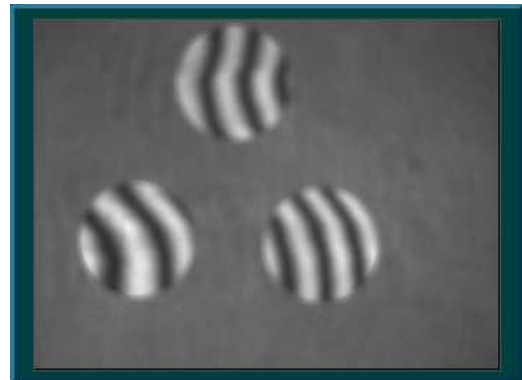
Figure 5. High orders modes linearity using Phase Diversity. Left: Comparison between differential high orders measurements on DWARF and by the ZYGO interferometer. Right: Interferogram obtained with the ZYGO.
