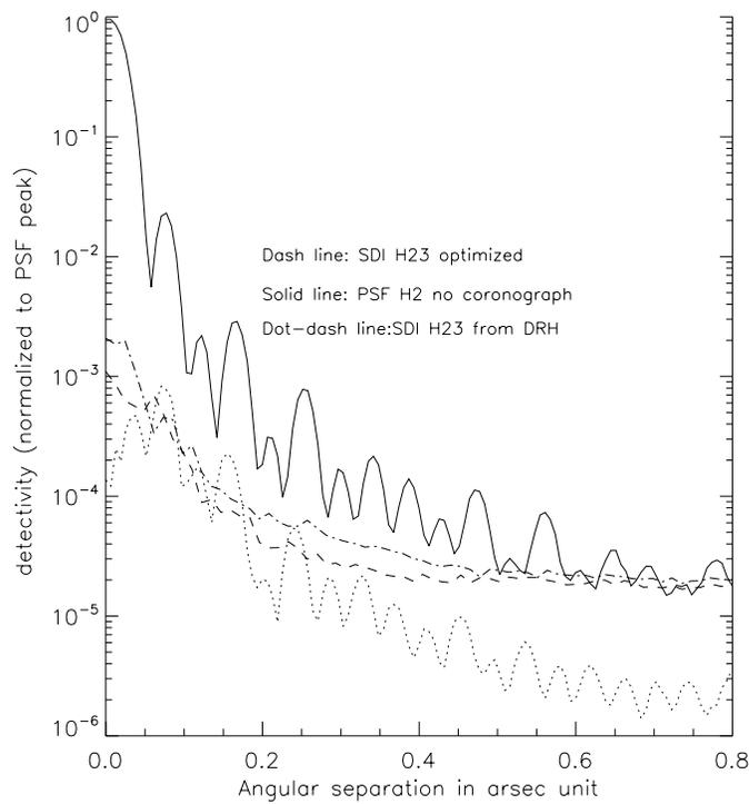
Figure 7: 5-sigma detection limits for the SDI applied on H2H3 data without coronagraph. The Dash line shows the achievable contrast while the solid line shows the H2 PSF.
