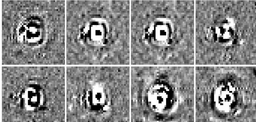
Figure 3: PSF speckle residual (taken for derotator positions ranging from 2 to 20 degrees) after subtracting the initial PSF (without derotation) at 1.6 microns.
