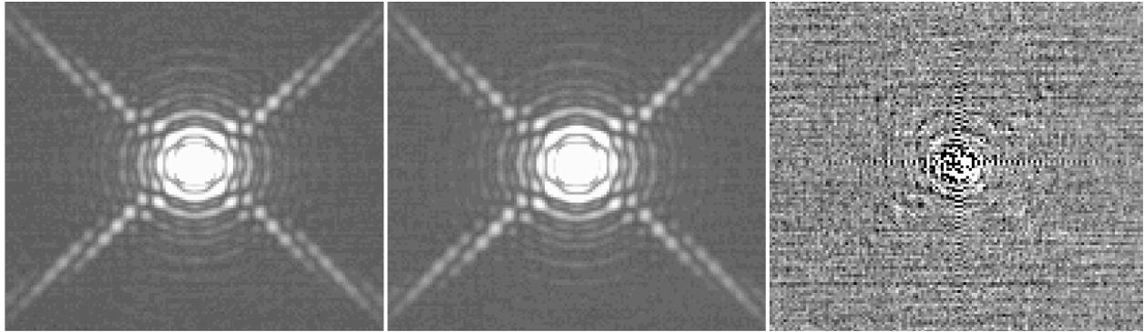
Figure 6: PSF obtained simultaneously thru H2 (Left) and H3 (Center) filters. The PSF residual (Right) obtained after spectral differential imaging.
