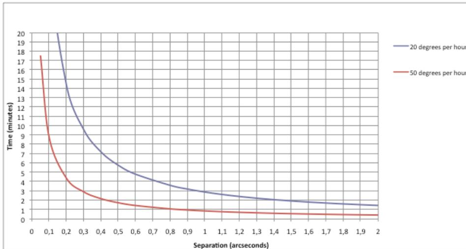
Figure 2: Time required to reach a field rotation of one pixel as function of the angular separation for 20 & 50 degree per hour field rotation rates.
