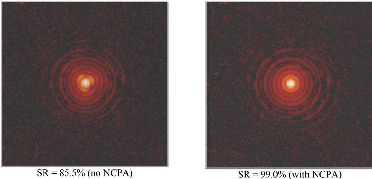
Figure 4: Both illustrations show the star PSF with and without non common path aberrations compensation
