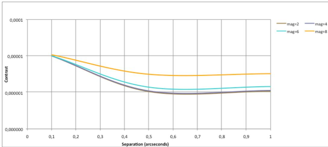
Figure 5: Expected contrast performance as function of stellar magnitude and angular separation
