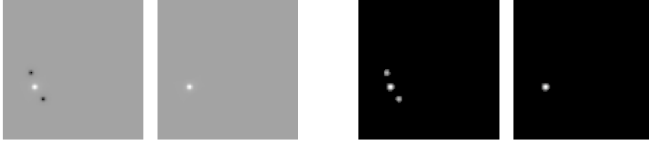
Fig. 2. Estimated flux map, without and with positivity constraint (1st and 2nd image) and corresponding J maps (3rd and 4th), for a theoretical noiseless case. We can remark the two sidelobes disappearing when the positivity constraint is applied.
