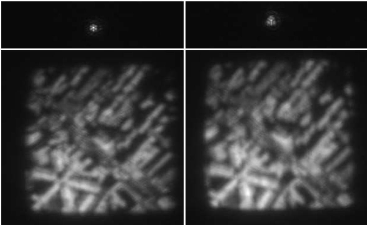
**Figure 4.** Focused (left) and defocused (right) experimental images of the extended scene (bottom) and reference point source (top).
