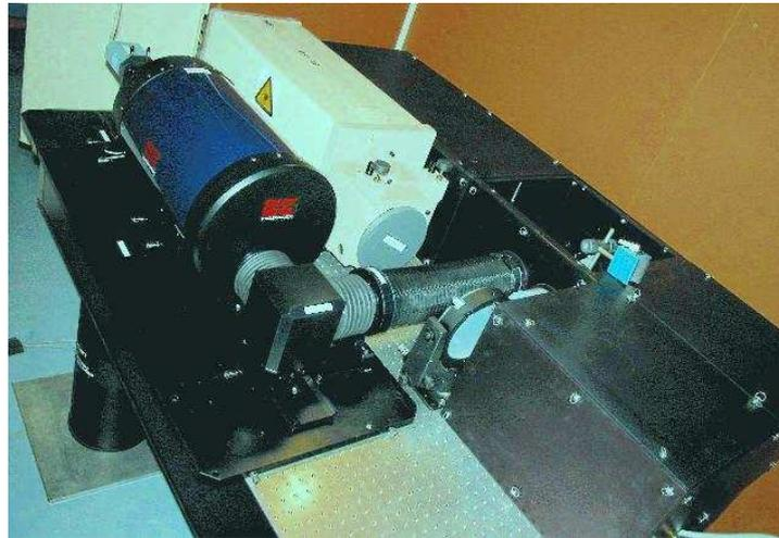
**Figure 8.** Photograph of BRISE (right side) with the Zygo interferometer (center) and the Darwin Fringe Sensor DWARF (left side) installed as a visitor instrument.
