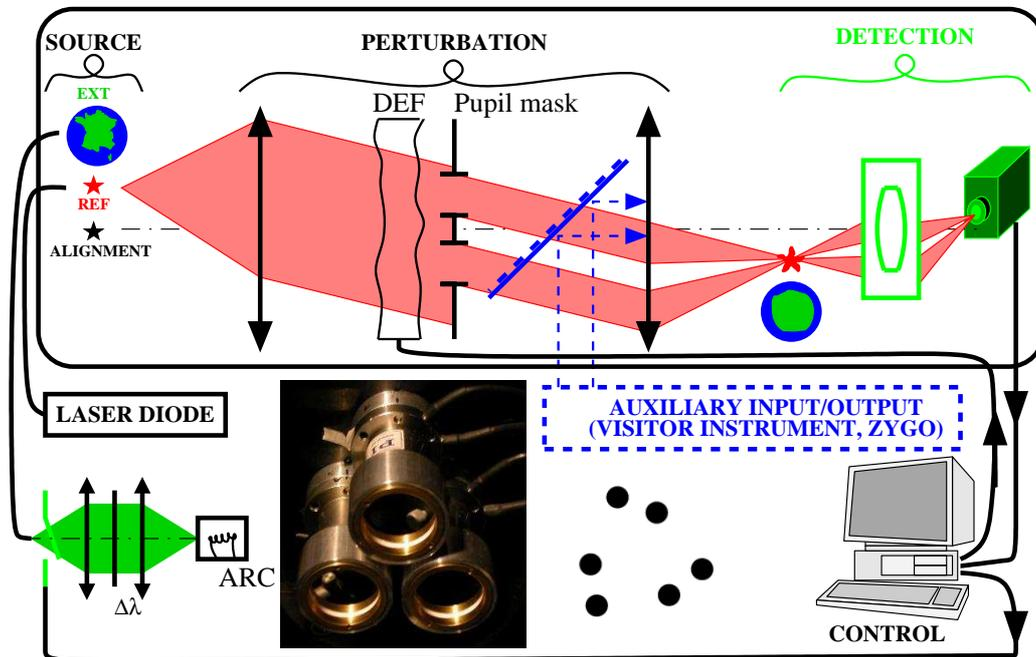
Figure 2. Schematic view of BRISE and photograph of the deformable mirror (DEF).
