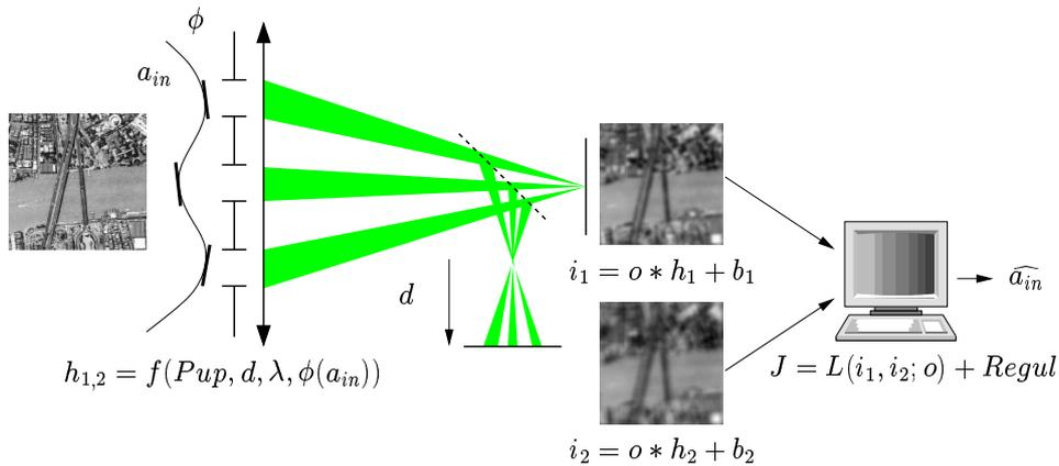
**Figure 1.** Principle of a Phase Diversity Sensor (PDS) implemented near a MAOT focal-plane.
