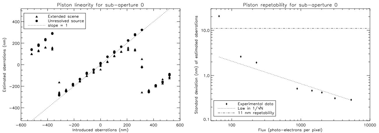
**Figure 7.** Piston measurements with the extended object. Left: Piston measured on the first sub-aperture, as a function of the piston introduced by the DEF. Right: Repeatability of the piston measured on the first sub-aperture, as a function of the average photon level per pixel.
