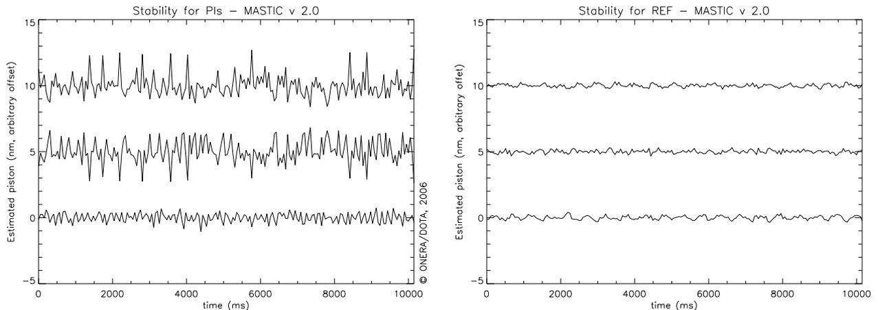
**Figure 6.** Temporal evolution of the differential piston for DEF mirror (left) and REF mirror (right).
