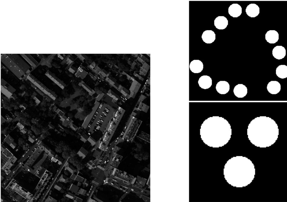
**Figure 3.** Left: extended scene used for simulations and experiments. Right: masks with 3 and 12 sub-apertures.
