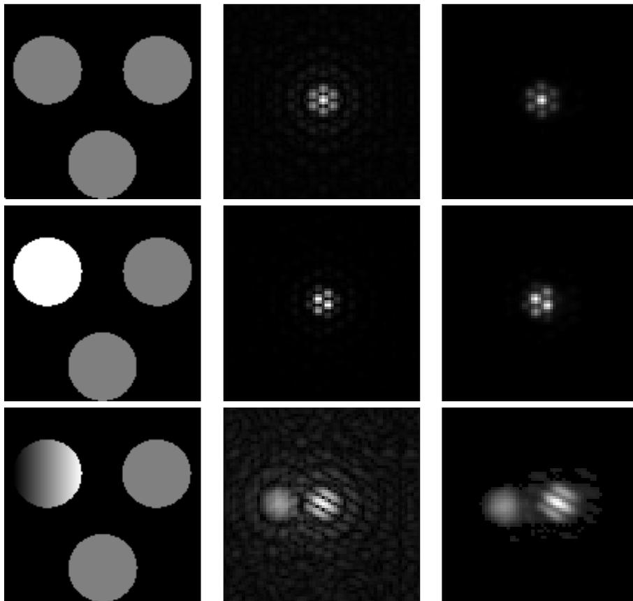
**Figure 5.** Agreement experimental results with BRISÉ (right column) and the direct model used for data processing with MASTIC (center column), in response to a given known phase perturbation (left column). *Cf text for details.*
