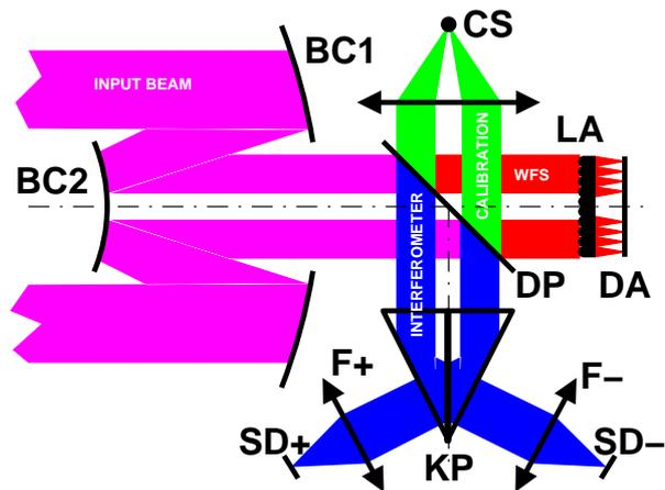
BC1+BC2:Beam Compressor ; LA:Lenslet Array ; DA:Detector Array ; CS:Calib. Source ; DP:Dichroic Plate ; KP:Koster Prism ;  $SD_{\pm}$ :Single-pixel Detector.
