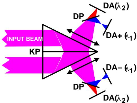
KP:Koster Prism ; DP: Dichroic Plate ;  $DA_{\pm}$ : Detector Array ; DA: tip/tilt Detector Array.
