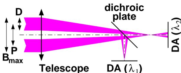
Figure 3. Concept ③: Focal-plane interferometer.
