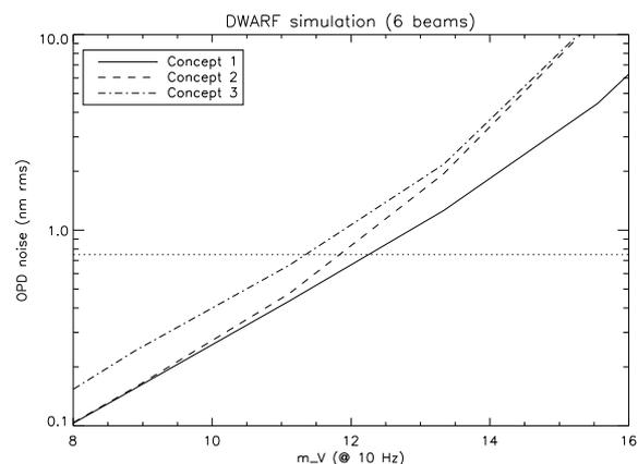
Figure 4. Simulated performance of the three setups. The dotted line is the specification. All the photons available in the  $V$  band ( $\lambda = 0.55 \mu\text{m}$ ,  $\Delta\lambda = 0.089 \mu\text{m}$ ) have been used (targets are characterized by their  $V$  magnitude).
