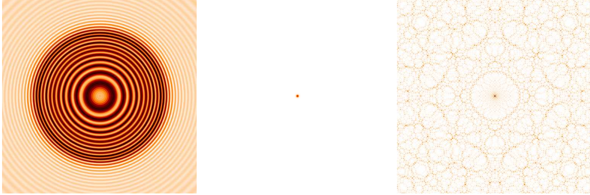
Fig. 1. Example of a defocused plane of the 3D PSF with the three imaging techniques we studied. Left : conoscopic holography; middle : classic imaging with a circular pupil; right : CSIG
