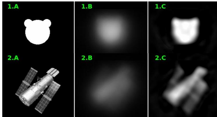
Fig. 2. Column A: original objects. Column B: frame number 1 of the blurred and noisy simulations. Column C: reconstructions: 1.C – 100 iterations, 2.C – 200 iterations. Images are represented on linear scale from 0 to 250.
